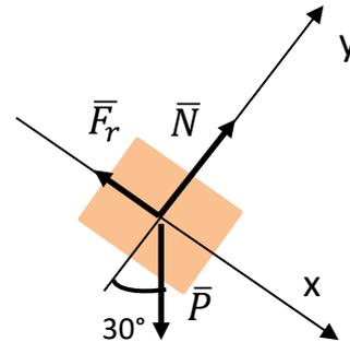
$$d) a = \frac{49 \text{N} - 7 \text{N}}{10 \text{kg}} = 4,2 \frac{\text{m}}{\text{s}^2}$$
